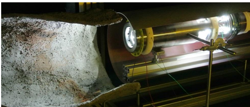
Figure 5: GeoKam prototype inside borehole model
