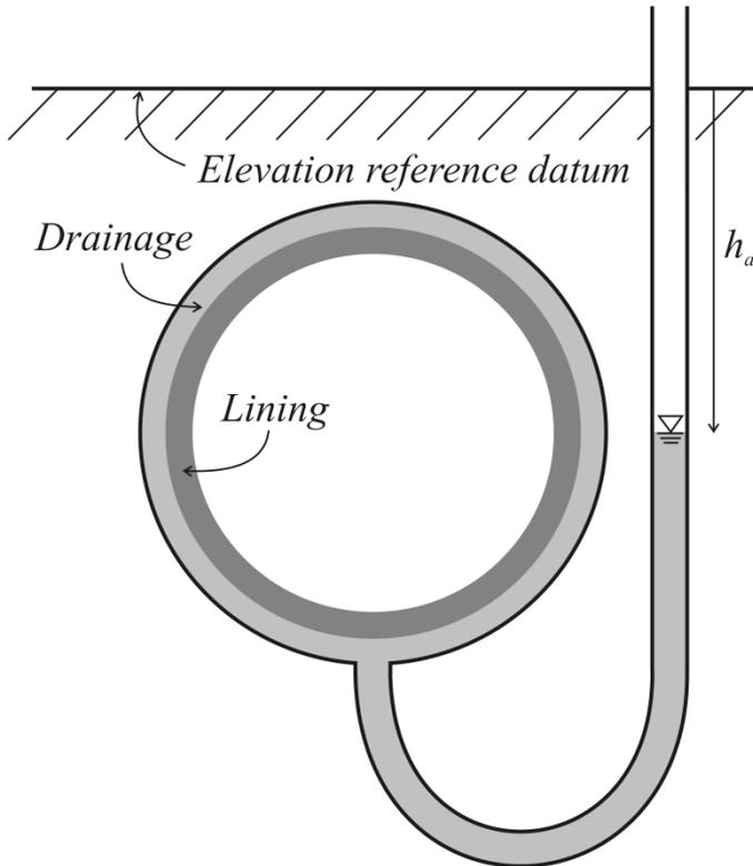
**Figure 1:** Drained tunnel with uniform hydraulic head  $h_a$  at tunnel perimeter.
