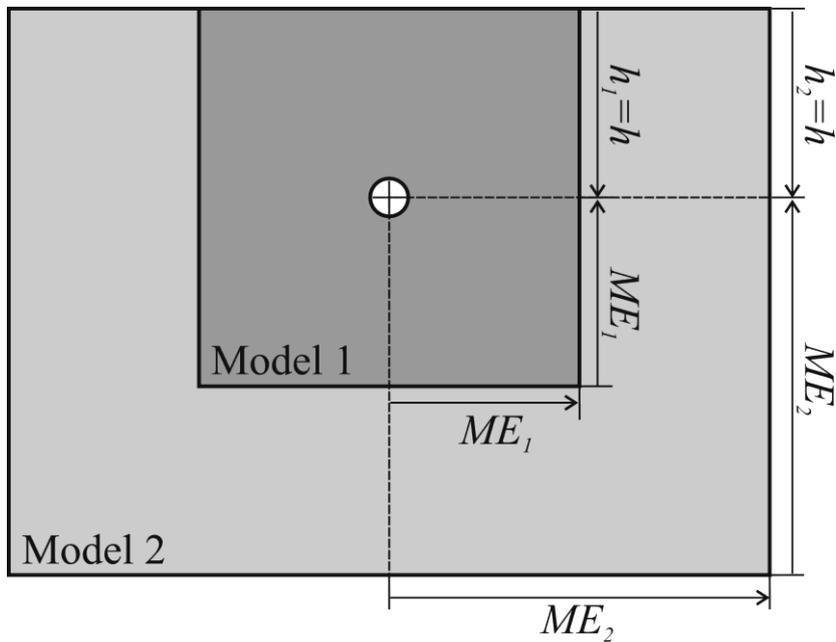
**Figure 4:** Depth of tunnel  $h$  and extent of model domain  $ME$  for two models with different  $ME$ . Subscripts refer to model 1 and 2.
