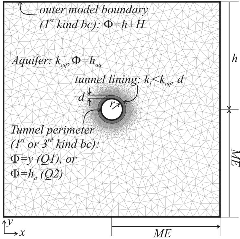
**Figure 3:** Finite element groundwater model with circular tunnel. Variables: see Table 2;  $h_a$ : also see Figure 1.
