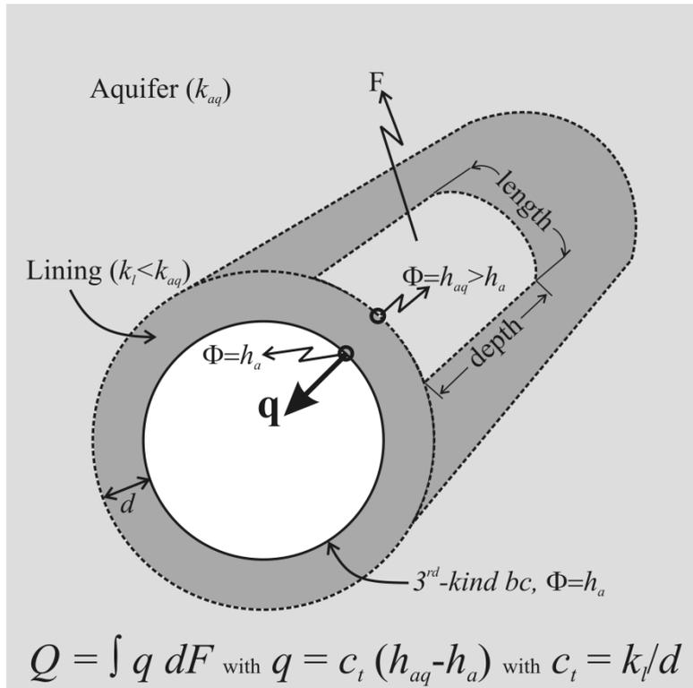
**Figure 5:** Calculation of tunnel inflow  $Q$  using a 3<sup>rd</sup>-kind BC, which includes specifying the hydraulic head (here:  $h_a$ ; c.f., Figure 1) and an outflow transfer rate  $c_t$  at the tunnel perimeter. Variables: see Table 2.
