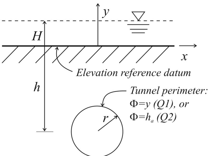
**Figure 2:** Circular tunnel in a semi-infinite aquifer (from: Park et al., 2008). Variables: see Table 2.
