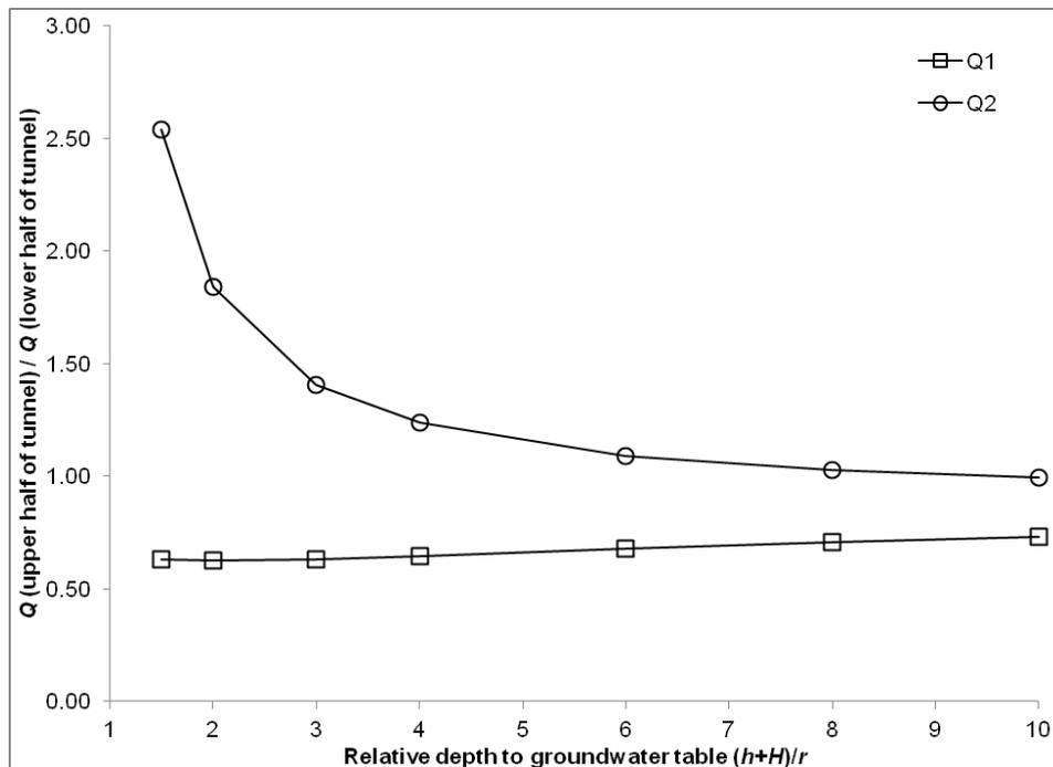
**Figure 10:** Inflow at upper half relative to the inflow at lower half of tunnel perimeter calculated for an unlined tunnel (type I) using an elevation head BC ( $Q1$ ) and for a lined tunnel with drainage layer (type II) using a uniform head BC ( $Q2$  with  $h_a = h$ ), plotted against the relative depth of the tunnel under the groundwater table.
