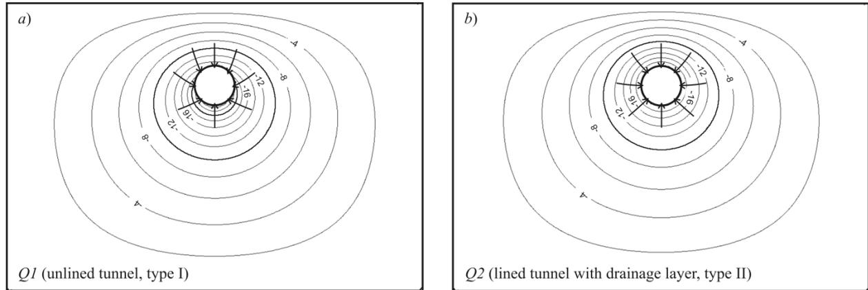
**Figure 11:** a) Distribution of hydraulic head in the aquifer and at the tunnel perimeter into an unlined tunnel (type I) using an elevation head BC ( $Q1$  with  $h = 4r$ ); and b) into a lined tunnel with drainage layer (type II) using a uniform head BC ( $Q2$  with  $h = 4r$  and  $h_a = h$ ).  $ME = 10r$ . Arrows indicate groundwater flow direction. Variables: see Table 2.
