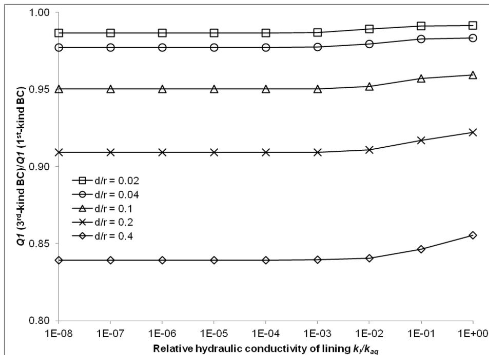
**Figure 12:** Difference between inflows  $Q1$  into lined tunnels without drainage layer calculated using a 1<sup>st</sup>-kind BC and a discretized lining (type IIIa) and using a 3<sup>rd</sup>-kind BC without discretizing the lining (type IIIb), plotted against the relative hydraulic conductivity of the lining ( $Q1$  using 3<sup>rd</sup>-kind BC normalized to  $Q1$  using 1<sup>st</sup>-kind BC). Different graphs represent different relative thicknesses of the lining.
