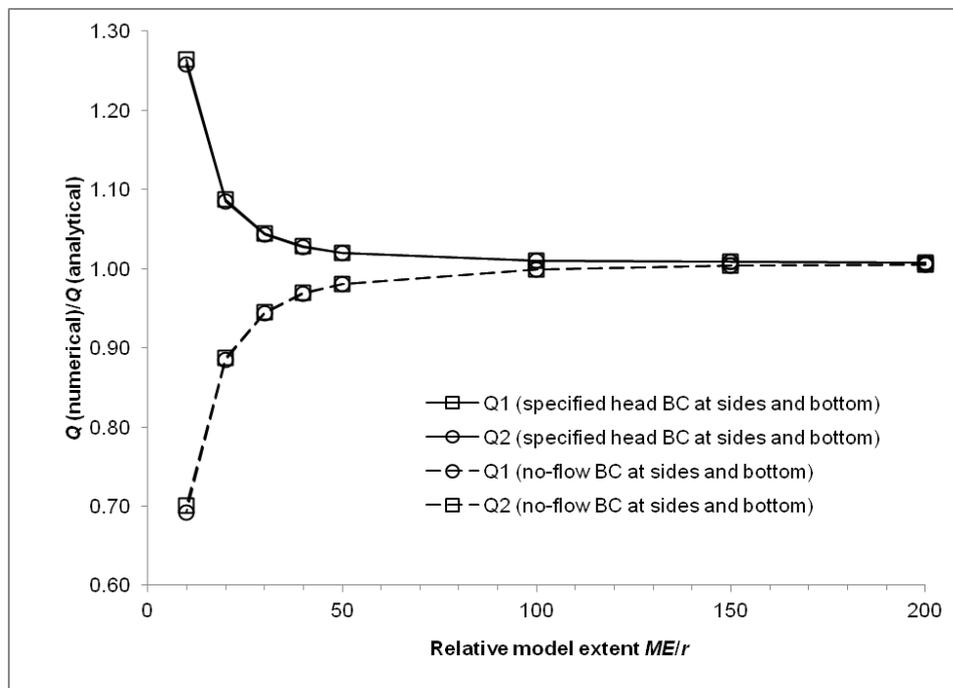
**Figure 6:** Difference between numerically and analytically calculated inflows into unlined tunnels (type I tunnels,  $Q1$ ) and into the drainage layer of lined tunnels (type II tunnels,  $Q2$ ) plotted against extent of model domain. Shown are numerical solutions  $Q1$  and  $Q2$  normalized to the analytical solutions (analytical solutions equal 1). At the lateral and bottom boundaries, either specified head BC (solid lines) or no-flow BC (dashed lines) are used in the numerical models.
