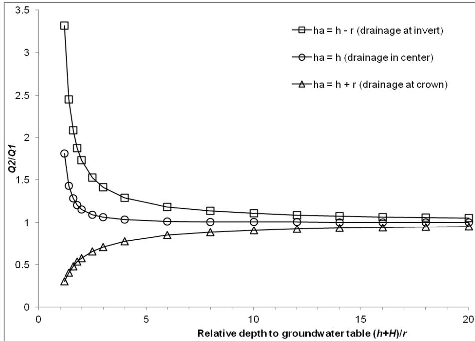
**Figure 9:** Difference between inflow  $Q1$  into unlined tunnels (type I) using an elevation head BC and inflow  $Q2$  into lined tunnels with drainage layer (type II) using a uniform head BC plotted against the relative depth of the tunnel under the groundwater table (analytical solutions; normalized to  $Q1$ ). Shown are solutions for different hydraulic heads  $h_a$  in the drainage layer of type II tunnels to calculate  $Q2$ .
